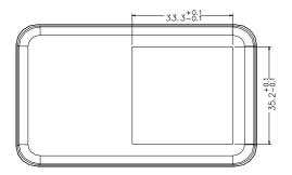
Other tolerances:±0.2mm Be connecting the wire W1 B O W2 and W3 of be marked text.
